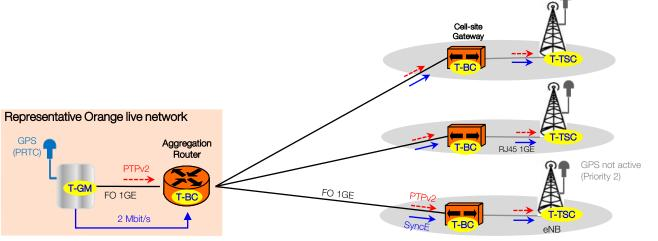
PRTC: Primary Reference Time Clock T-GM: Telecom Grandmaster T-BC: Telecom Boundary Clock T-TSC: Telecom Time Slave Clock
