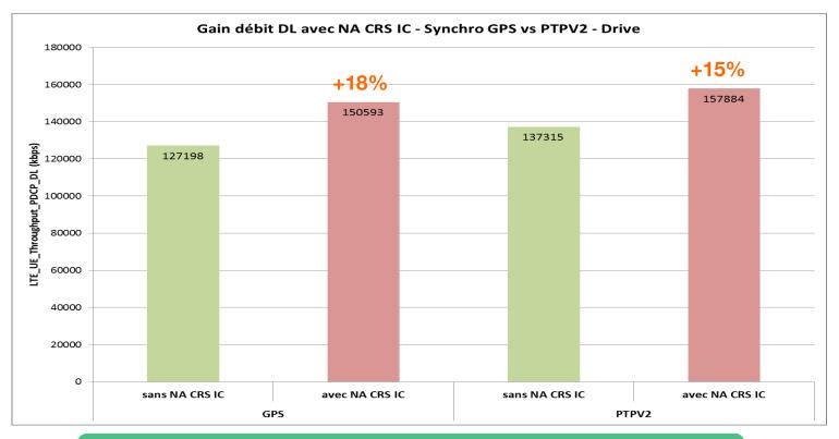
Similar (better!) gain with NA CRS IC feature with GPS or PTPv2 synchronization
